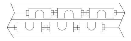
The rollers should be positioned so that the openings face each other. They slide onto the end of the top frame piece, at the ends, prior to the affixing of the panels.
